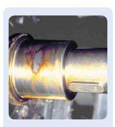
SKF LGAF 3E prevent fretting corrosion caused by very slight oscillations or by vibrations, that can make dismounting much more difficult.
